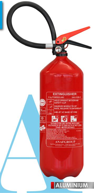
PS6-J ABC is a stored pressure, multi-purpose dry powder fire extinguisher with pressure gauge. Wide operating temperature range -30 °C +60 °C, ensuring suitability for use in low-temperature countries. Certified to the Pressure Equipment Directive PED 2014/68/EU, to the Marine Equipment Directive MED 2014/90/EU and CEN EN3-7. 100% of the fire extinguishers are checked by an electronic helium leak detection system.
