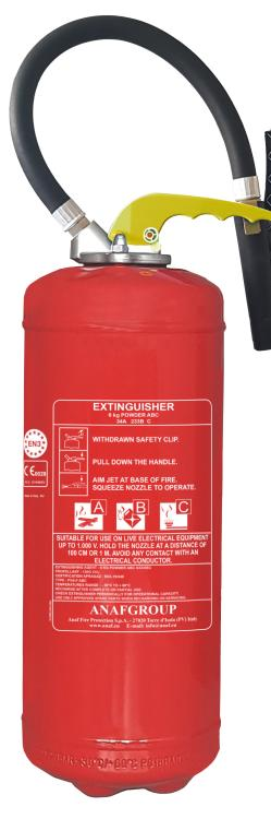
PG6-F ABC is an auxiliary pressure powder fire extinguisher with mild steel body. Certified according to the Pressure Equipment Directive PED 2014/68/EU Capacity is 6 Kg.
