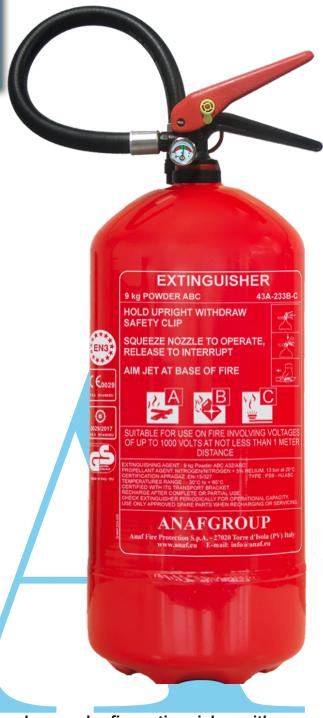
PS9-HJ ABC is a stored pressure, multi-purpose dry powder fire extinguisher with pressure gauge. Wide operating temperature range -30 °C +60 °C, ensuring suitability for use in low-temperature countries.
