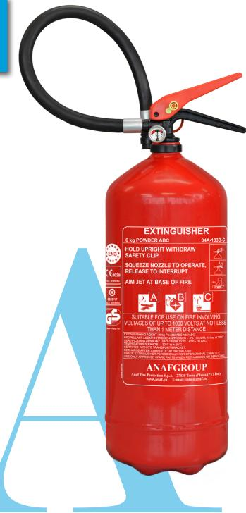
PS6-HJ ABC is a stored pressure, multi-purpose dry powder fire extinguisher with pressure gauge. Wide operating temperature range -30 °C +60 °C, ensuring suitability for use in low-temperature countries. Certified to the Pressure Equipment Directive PED 2014/68/EU, to the Marine Equipment Directive MED 2014/90/EU and EN3-7. 100% of the fire extinguishers are checked by an electronic helium leak detection system.
