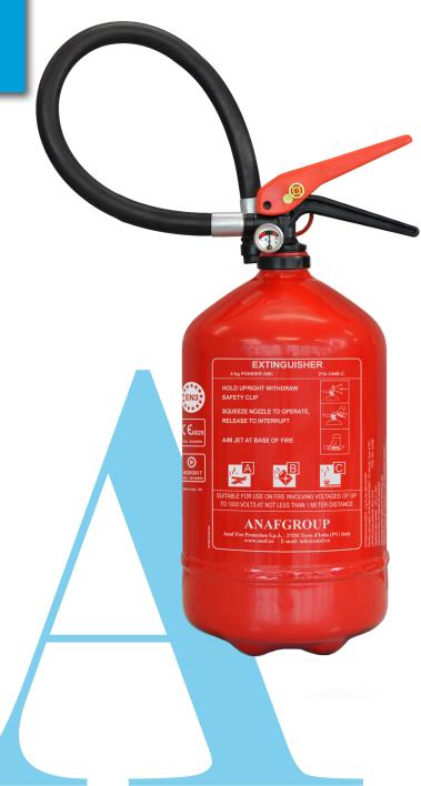
PS4-HJ ABC is a stored pressure, multi-purpose dry powder fire extinguisher with pressure gauge. Wide operating temperature range –30 °C +60 °C, ensuring suitability for use in low-temperature countries. Certified to the Pressure Equipment Directive PED 2014/68/EU, to the Marine Equipment Directive MED 2014/90/EU and EN3-7. 100% of the fire extinguishers are checked by an electronic helium leak detection system.
