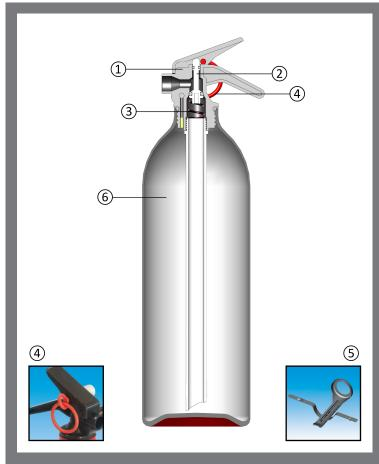
1 The valve is made up of acetal resin ensuring perfect corrosion protection.
