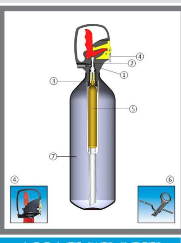
(1) The valve is made up of acetal resin ensuring perfect corrosion protection.
