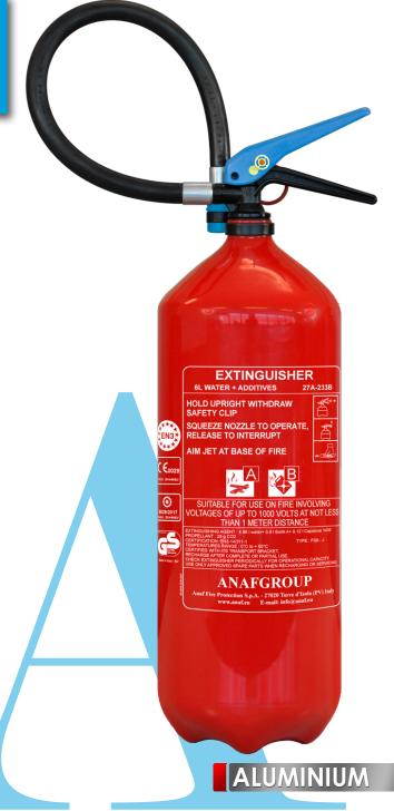
FG6-J is an auxiliary pressure, spray foam fire extinguisher with aluminium body. Certified to the Pressure Equipment Directive PED 2014/68/EU, Marine Equipment Directive MED 2014/90/EU and CEN EN3. Capacity is 6 l.
